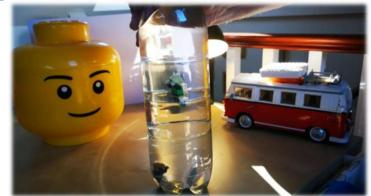
It is **Pascal's Law** that tells us that a change in pressure is felt within the entire bottle, including on the air bubble in the straw, and it is that increased pressure which compresses or forces the air bubble into a smaller volume inside the straw.....which makes our diver more **Dense.**
